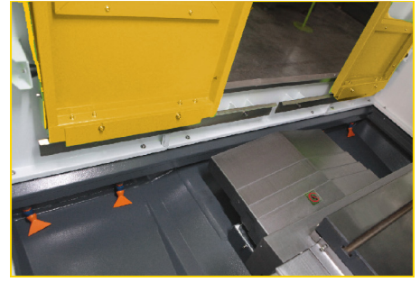
Chip flushing system
