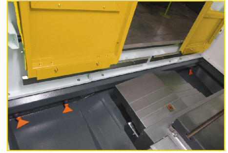
Chip flushing system
