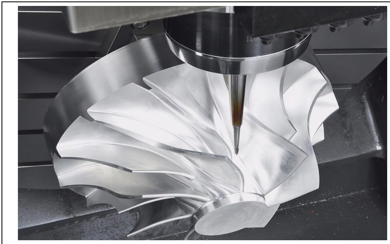
Crane-type High-Level 5 Axis Machining Centre The most advanced Direct drive spindle can handle high speed tooling to carry out economical and accurate machining by direct drive to the Rotary C-Axis and tilt A-Axis.
