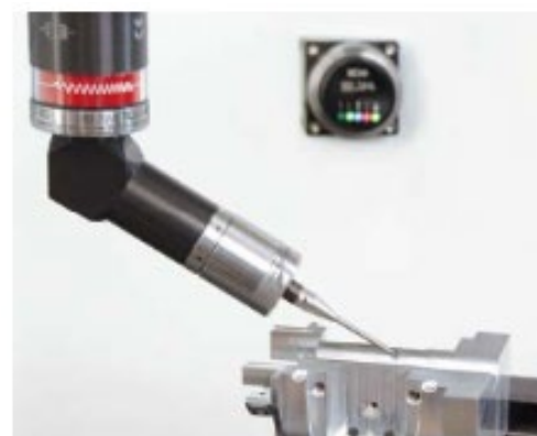
TC63-RG – modular system with shark360 DIGILOG technology
