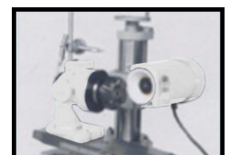
Sharpening face milling cutter being held in the C2SF fixture with arbor cutter, indexed with universal tooth rest and diamond cup wheel.
