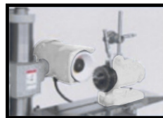
Sharpening side milling cutter held on C2Sh fixture with arbor. Plain tooth rest is indexed against index disc.
